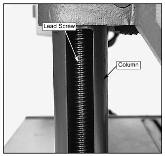
Figure 42. Lead Screw inside of column.
